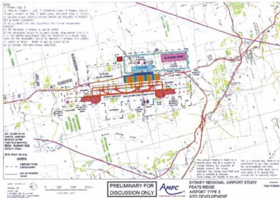
Figure 11 Peats Ridge Site - Preliminary Site Development for Type 3 Airport (Ref: Joint Study on aviation capacity in the Sydney region, Australia Govt / NSW Govt, March 2012. Technical Papers Vol.4, Appendix 3 – Concept Plans )
