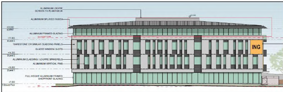
Figure 9. South elevation showing height control
