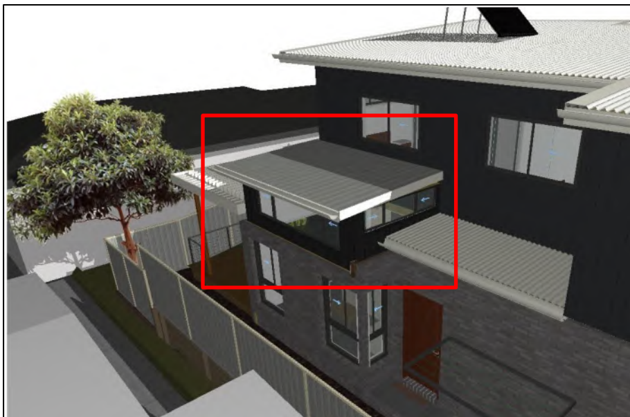
Figure 18 – solar access to Unit 3 at June 21, 12pm – raised roof over living area highlighted in red
