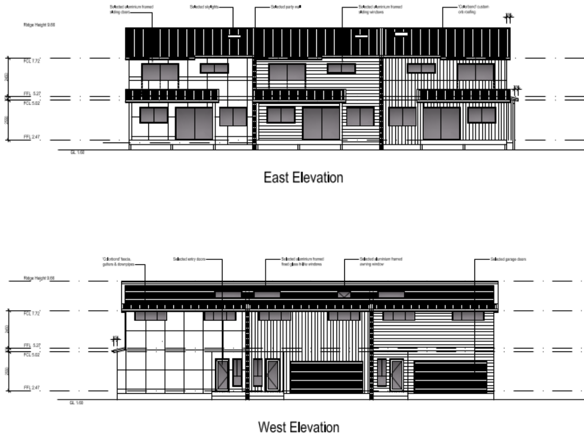
Figure 19 – East and West Elevations of Units 3, 4 and 5
