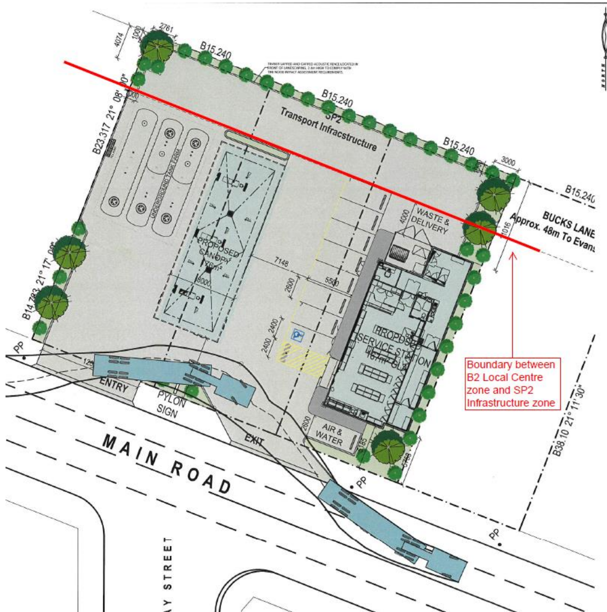
Figure 3 – Site Plan (a condition of consent is recommended requiring the acoustic fencing to be located within the B2 land and returning along part of the eastern and western boundaries).
