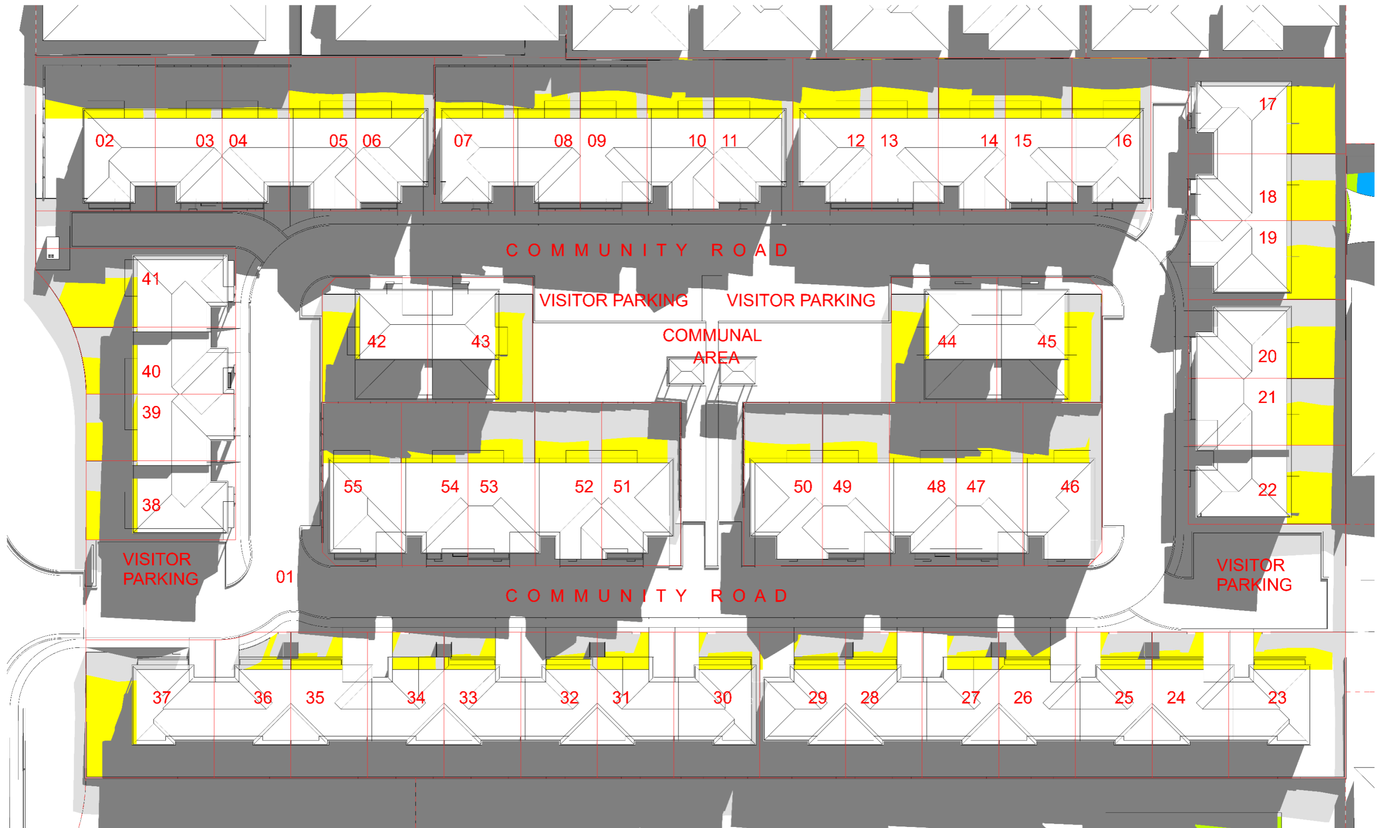
FIGURE 2 Shadow Diagram at Ground Level of Proposed Development at 10:00am on 21st June
