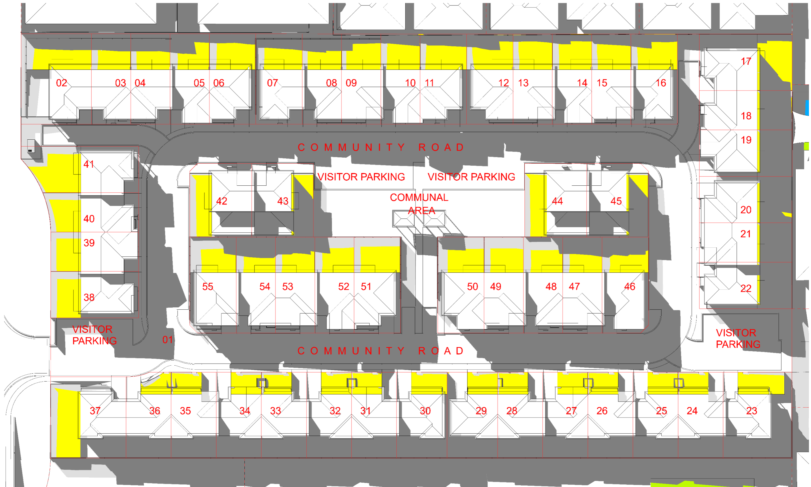
FIGURE 13 Shadow Diagram at 1m Above Private Open Space of Proposed Development at 2:00pm on 21st June
