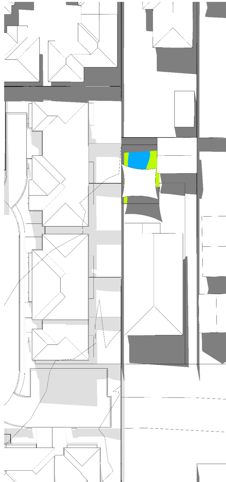
FIGURE 18 Shadow Diagram at Existing & Proposed Development at 12:00pm on 21st June at No.9 Oak Road
