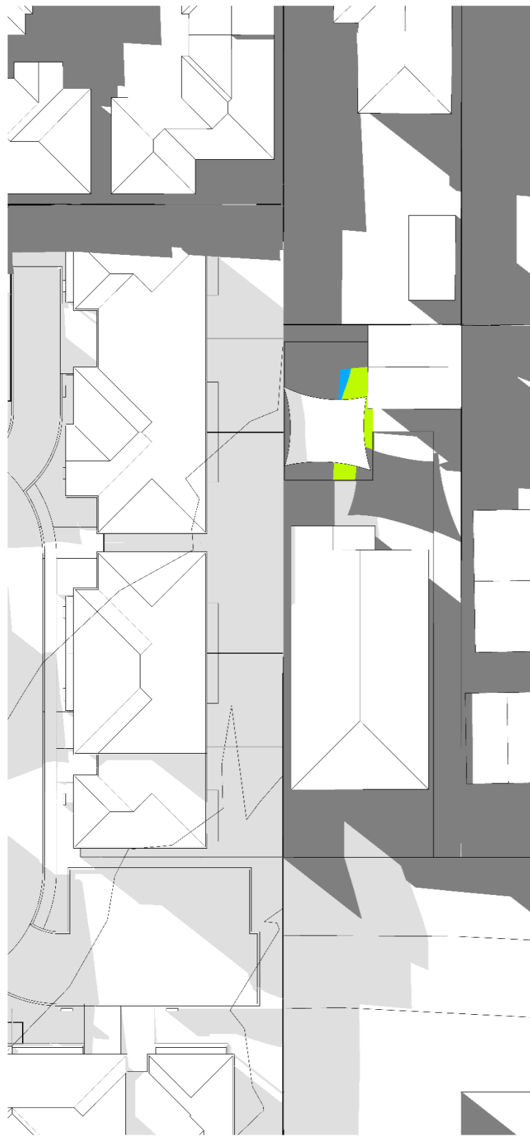
FIGURE 21 Shadow Diagram at Existing & Proposed Development at 3:00pm on 21st June at No.9 Oak Road
