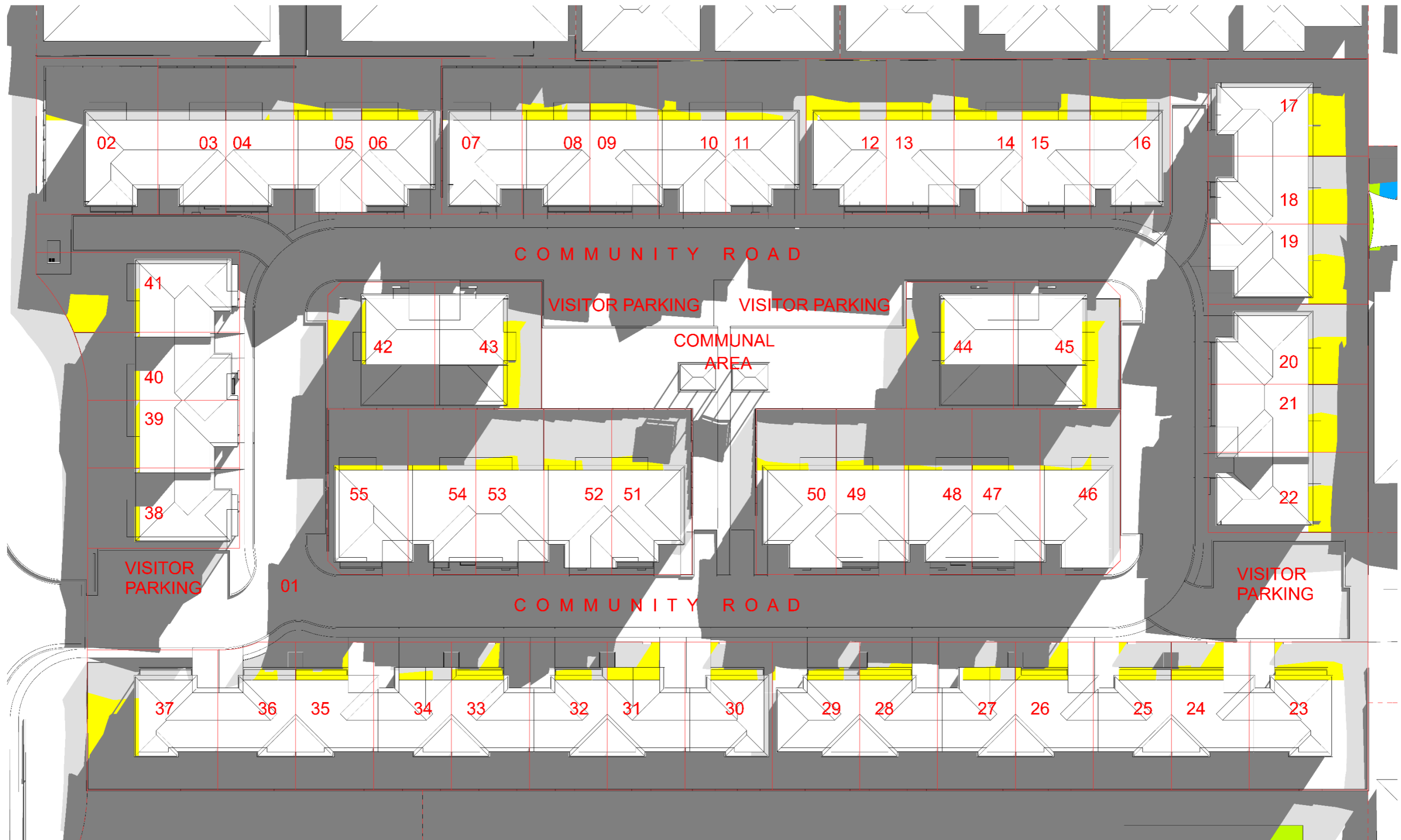
FIGURE 1 Shadow Diagram at Ground Level of Proposed Development at 9:00am on 21st June
