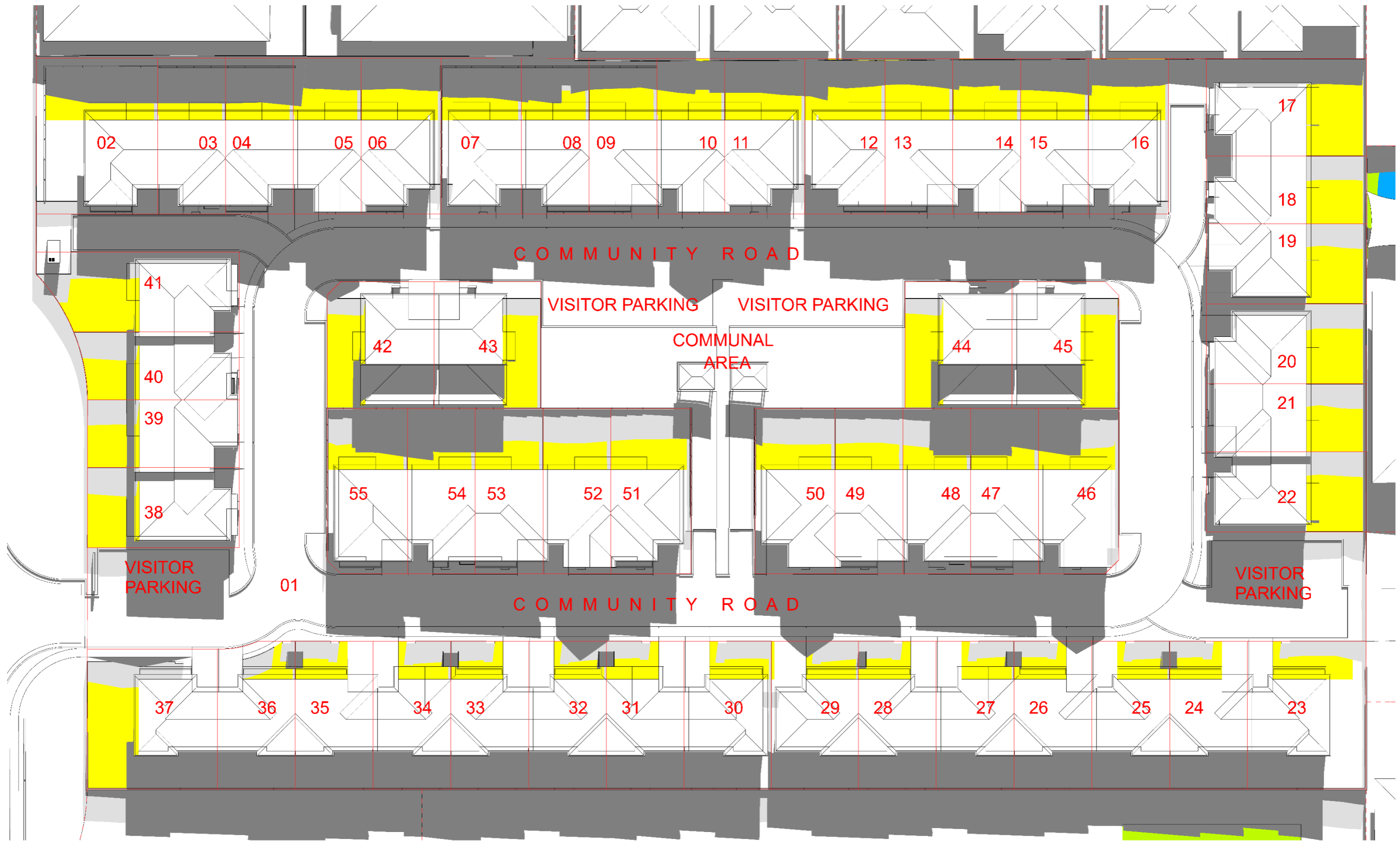
FIGURE 3 Shadow Diagram at Ground Level of Proposed Development at 11:00am on 21st June
