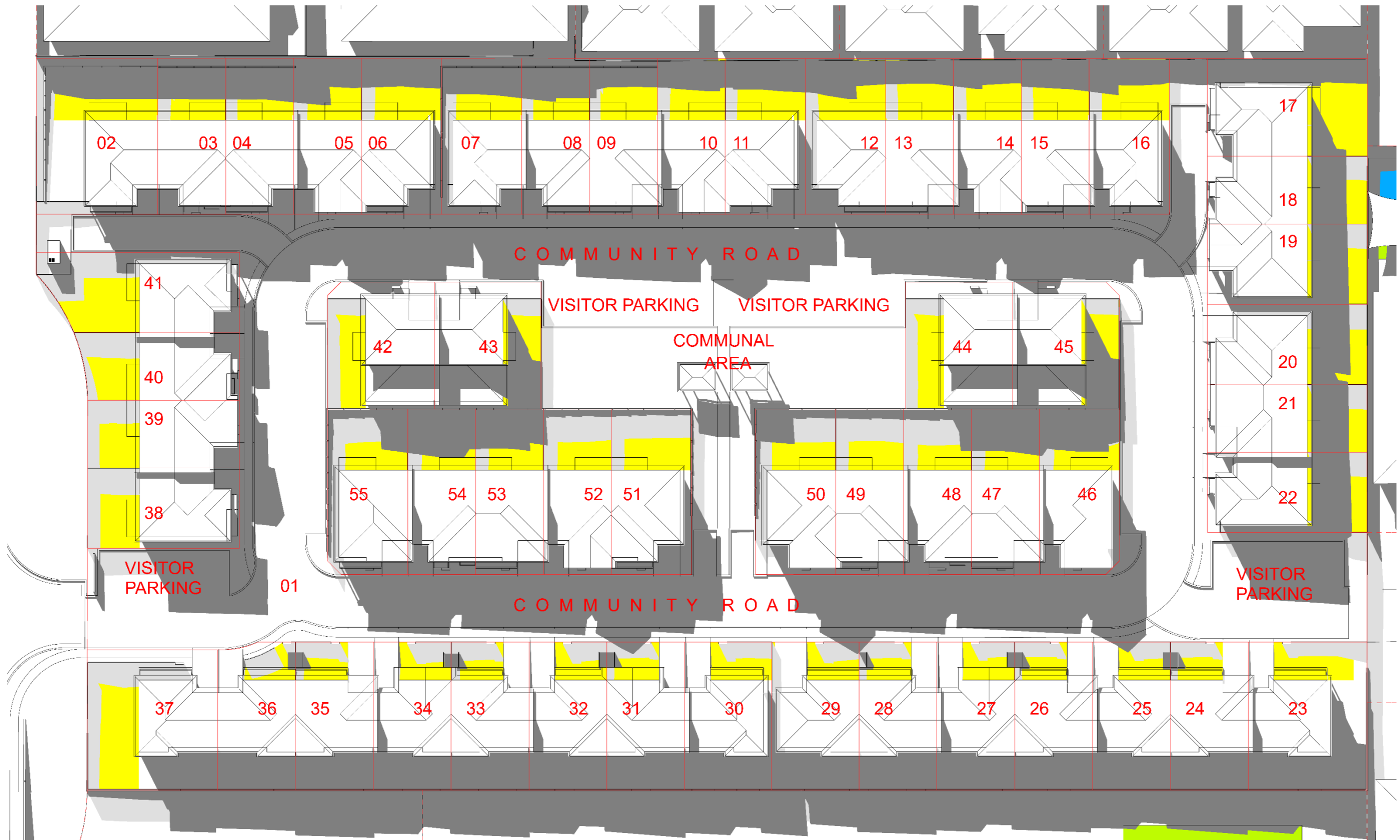
FIGURE 5 Shadow Diagram at Ground Level of Proposed Development at 1:00pm on 21st June
