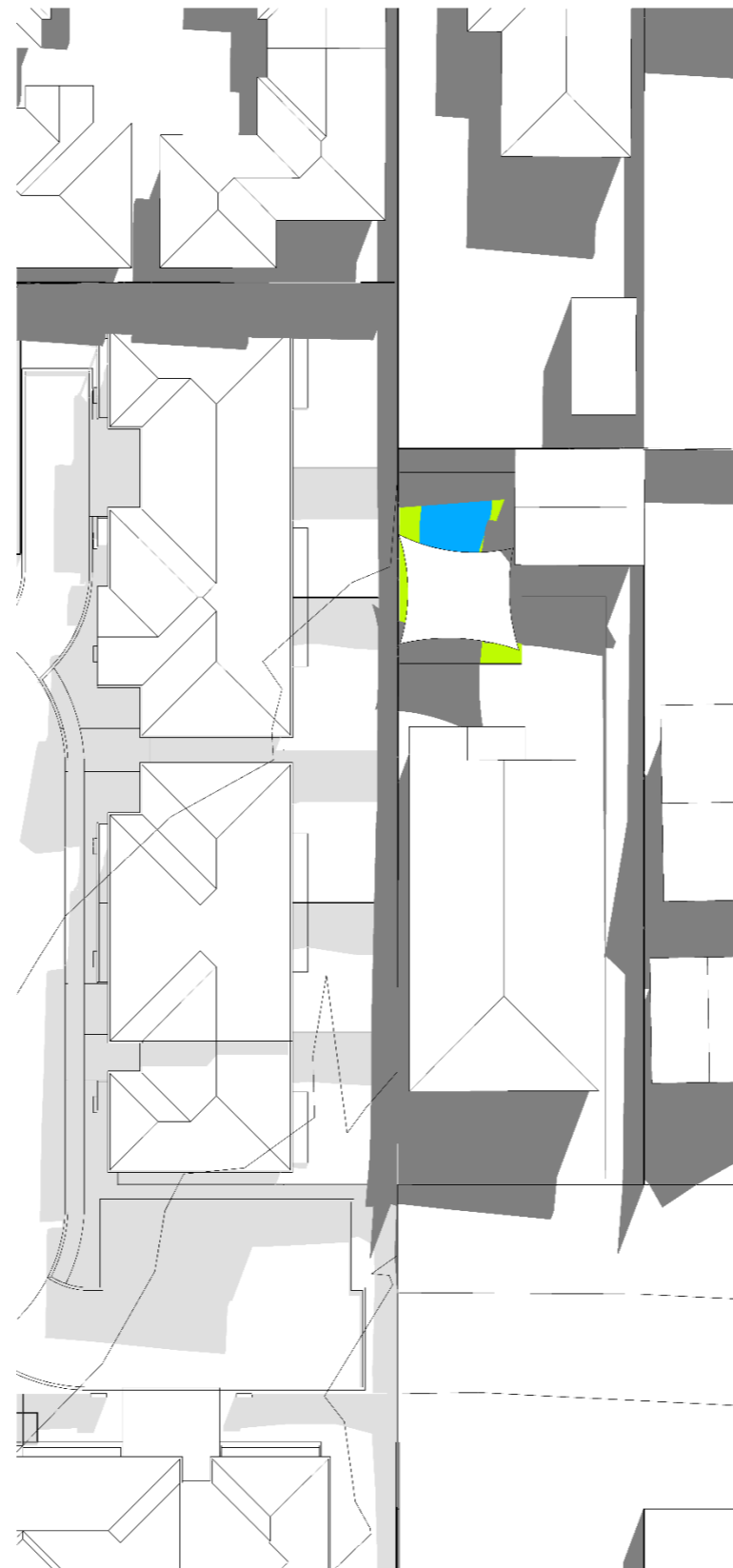
FIGURE 16 Shadow Diagram at Existing & Proposed Development at 10:00am on 21st June at No.9 Oak Road
