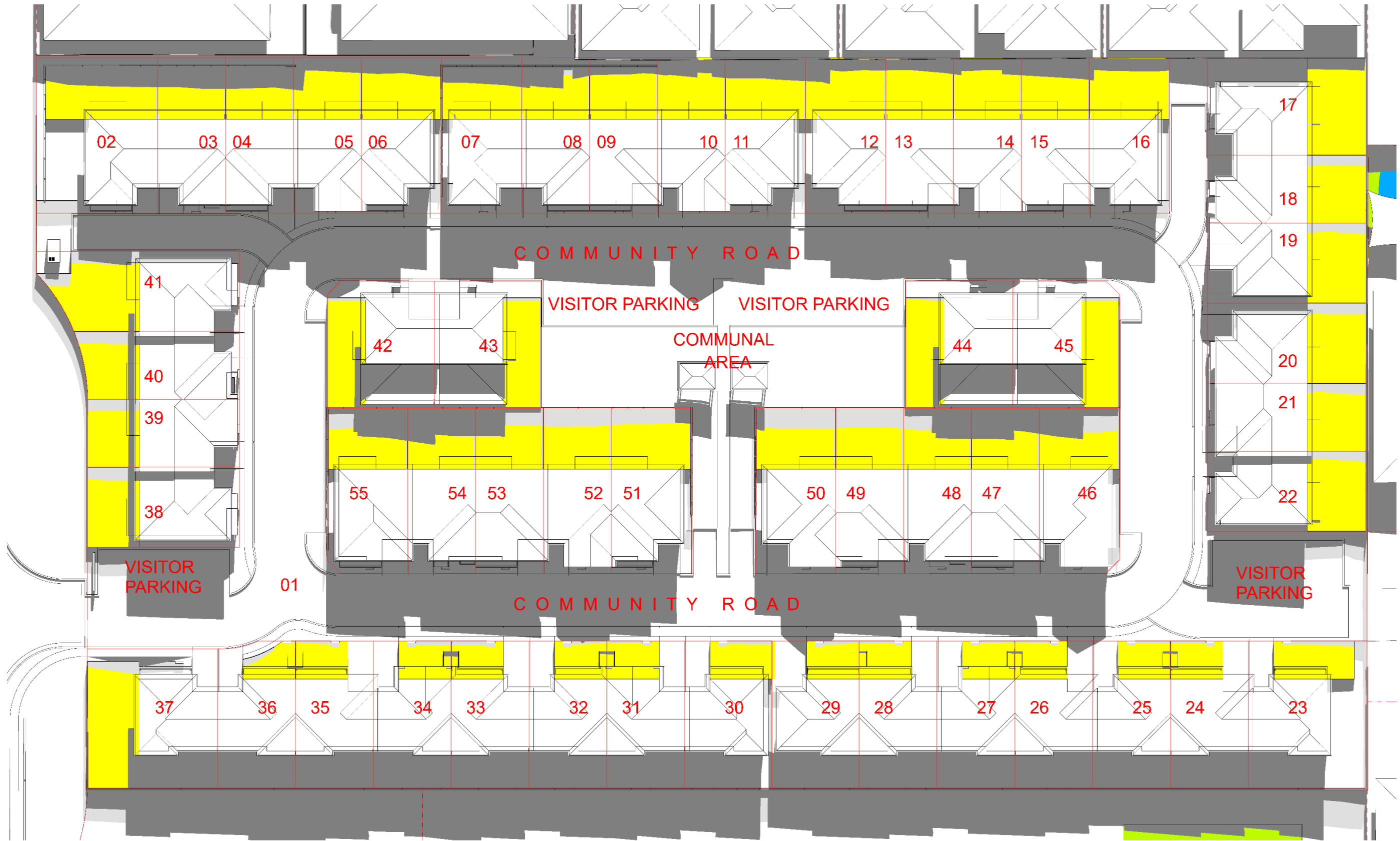
FIGURE 10 Shadow Diagram at 1m Above Private Open Space of Proposed Development at 11:00am on 21st June
