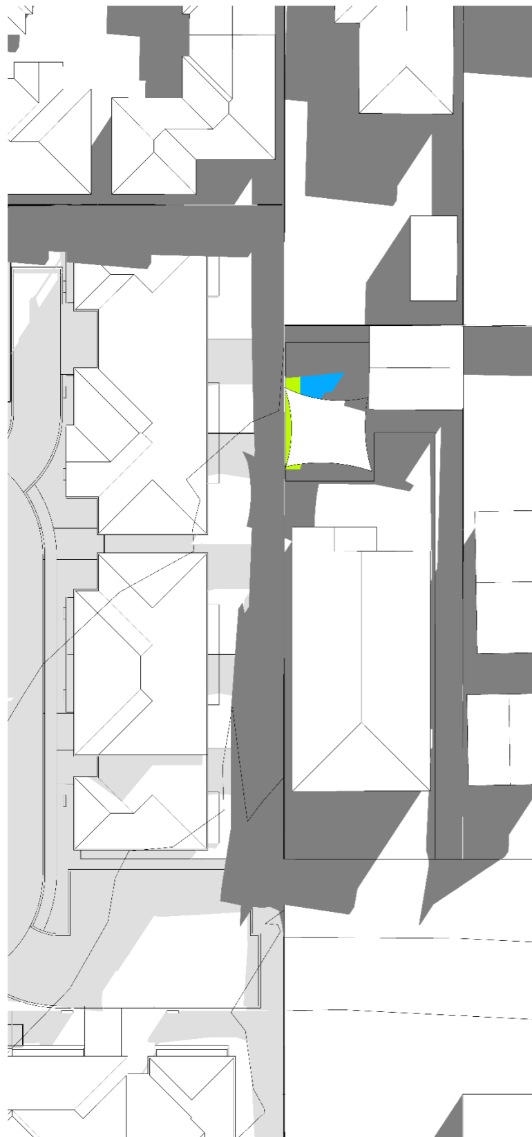
FIGURE 15 Shadow Diagram at Existing & Proposed Development at 9:00am on 21st June at No.9 Oak Road
