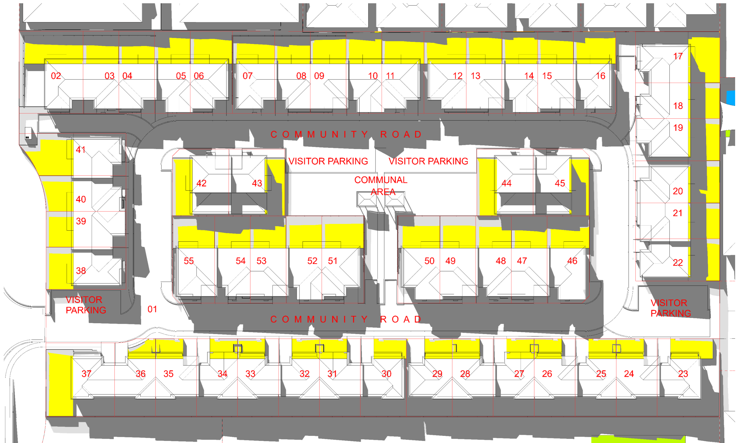
FIGURE 12 Shadow Diagram at 1m Above Private Open Space of Proposed Development at 1:00pm on 21st June
