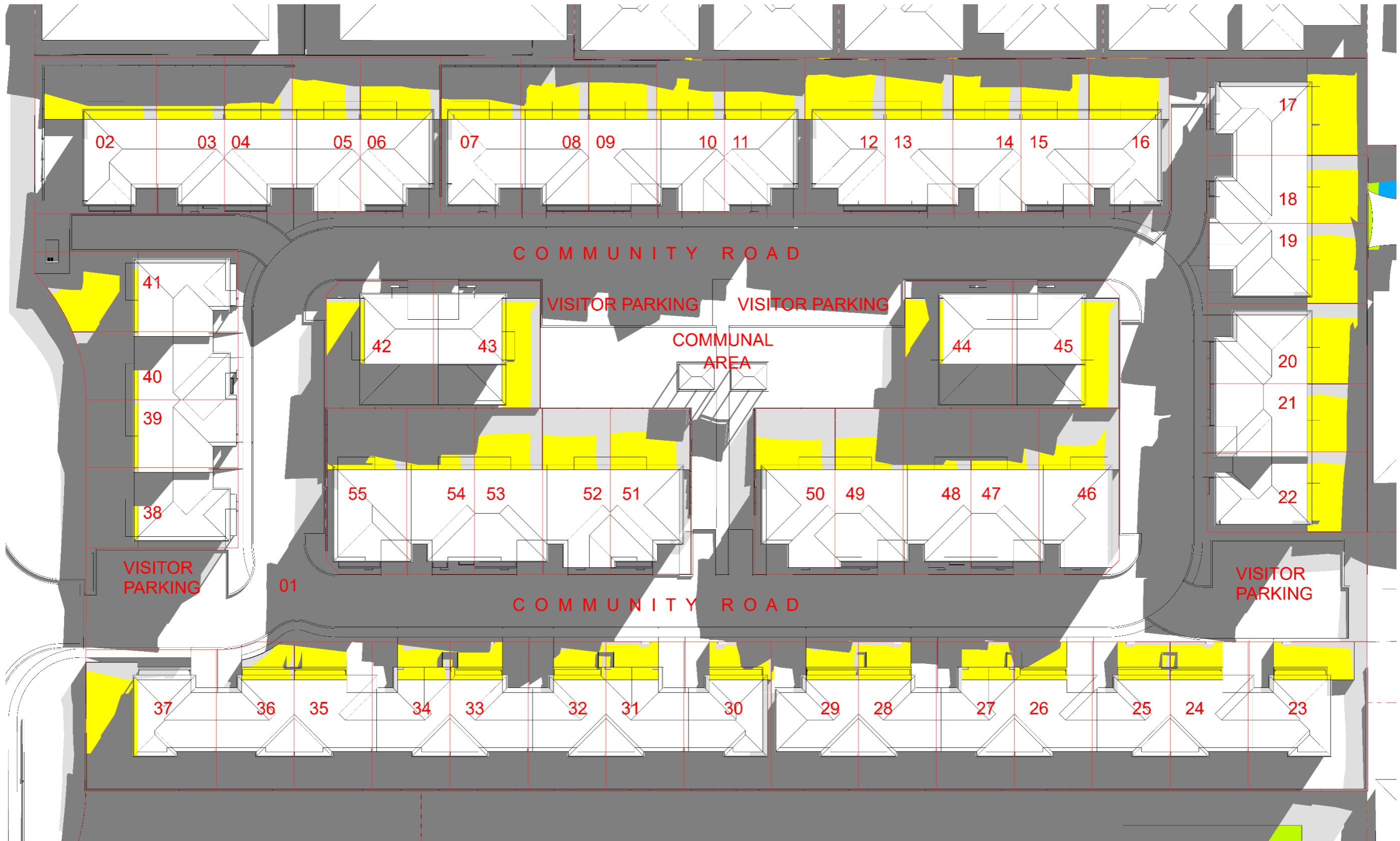
FIGURE 8 Shadow Diagram at 1m Above Private Open Space of Proposed Development at 9:00am on 21st June
