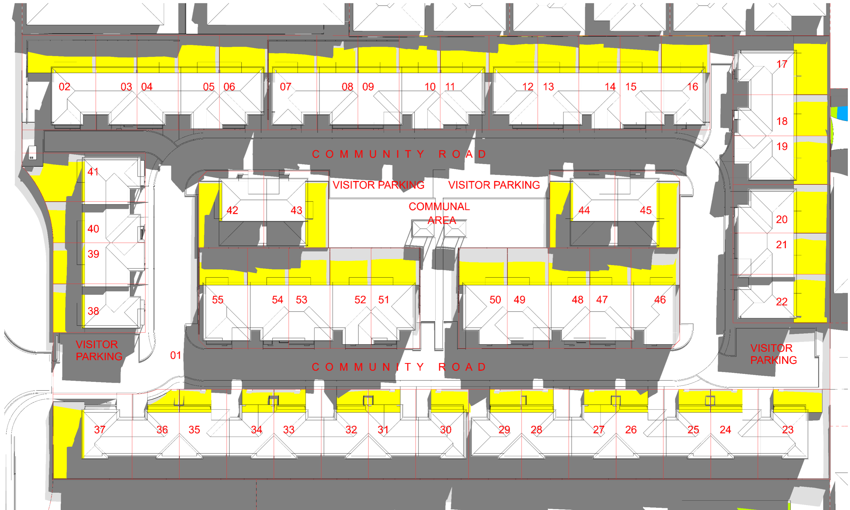
FIGURE 9 Shadow Diagram at 1m Above Private Open Space of Proposed Development at 10:00am on 21st June
