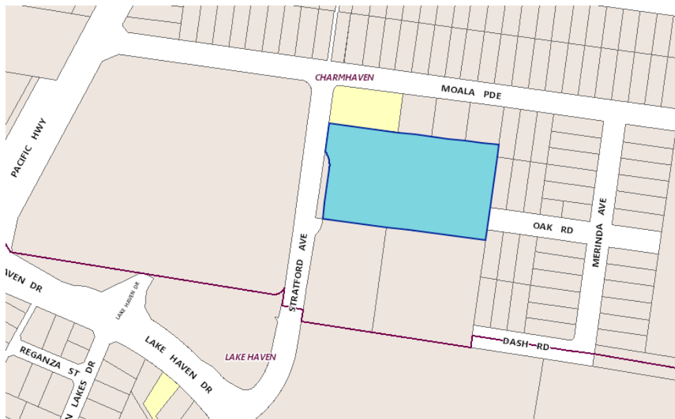
Figure 2 – Cadastral plan showing road network in vicinity of site (note: the portion of Stratford Avenue fronting the development site is currently unformed)
