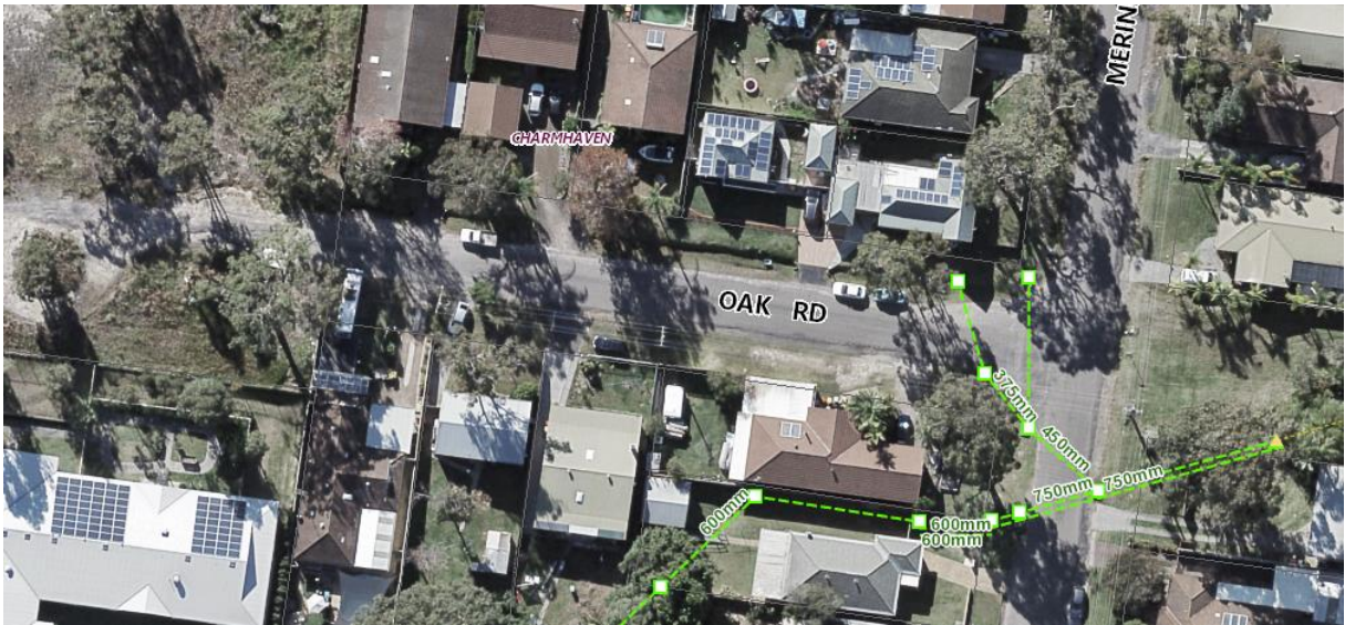
Figure 7 – Aerial photograph depicting existing downstream drainage infrastructure at the intersection of Oak Road / Merinda Avenue
