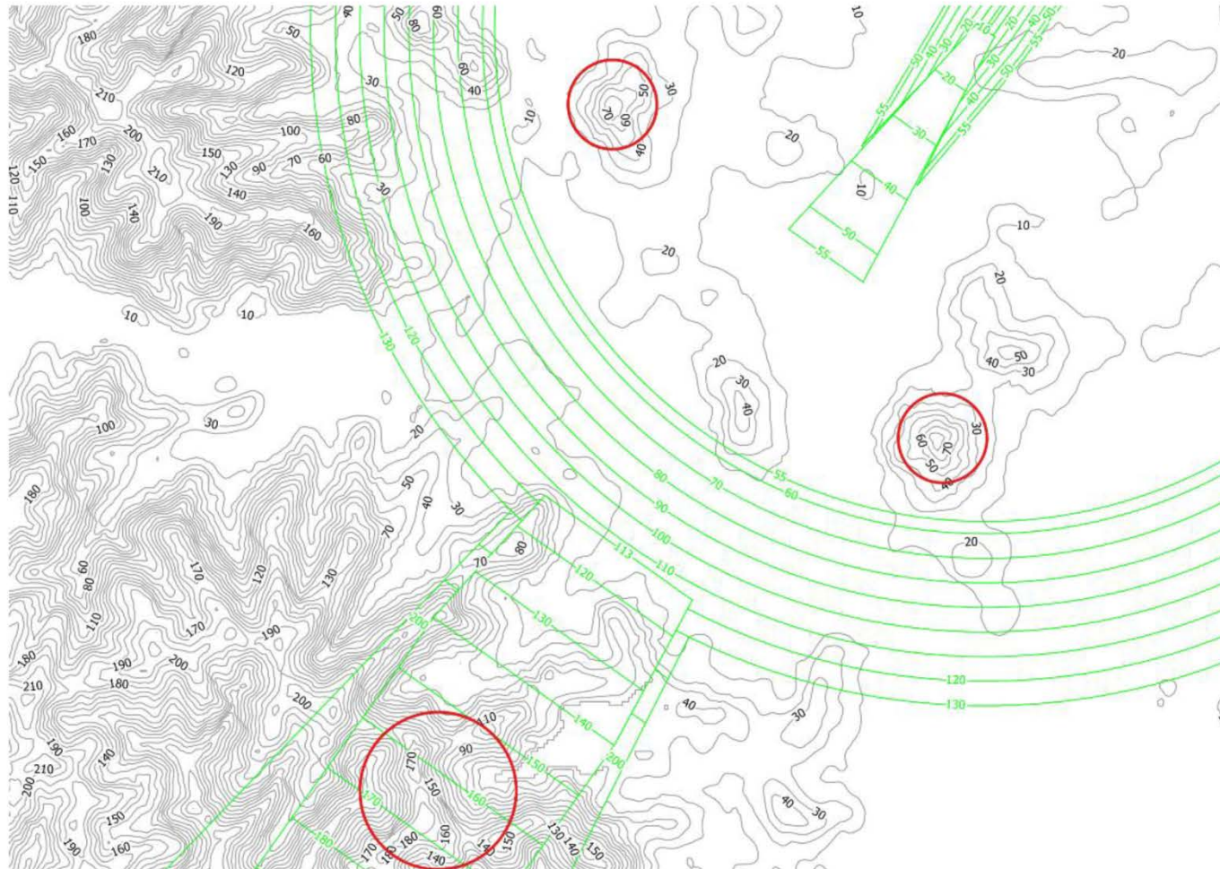
Figure 24 - 1200m RWY OLS terrain intrusions (a)
