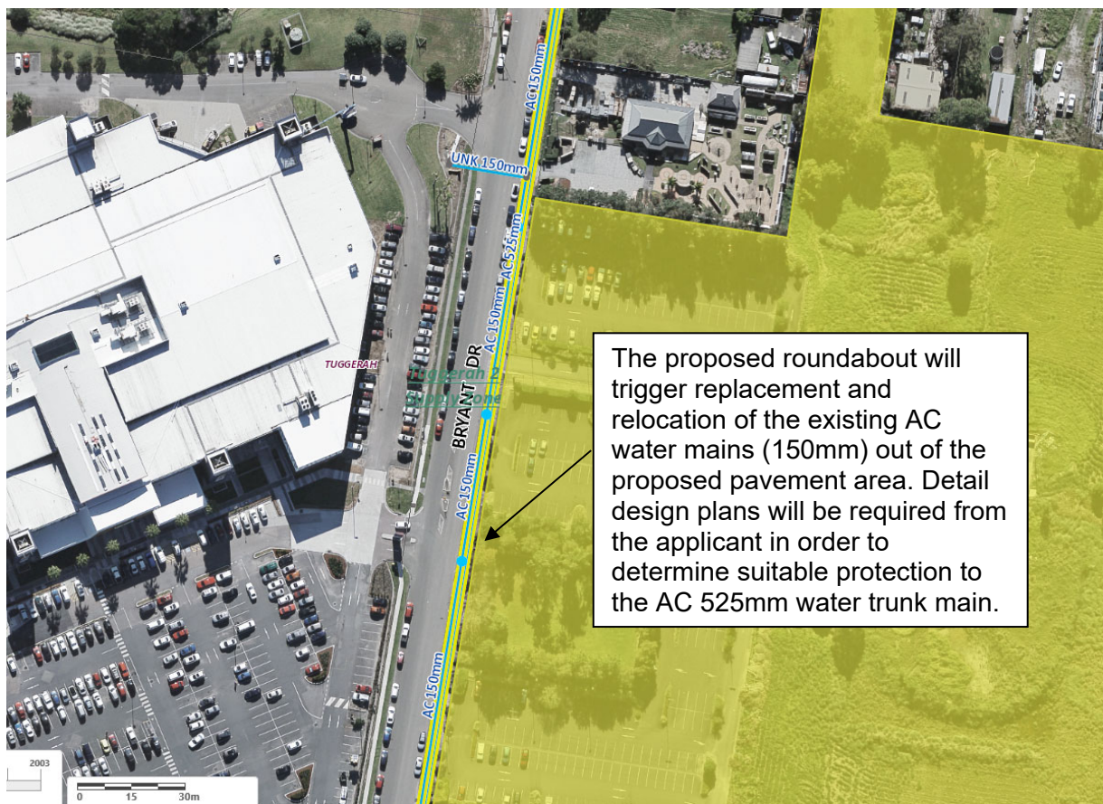
Figure 5: Water Supply Arrangements
