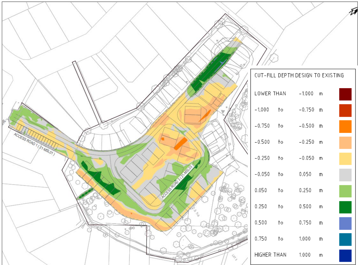
Figure 19: Earthworks Cut and Fill Plan
