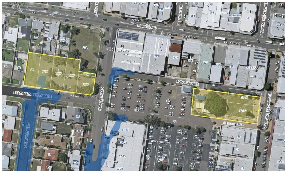
Figure 5 - Flood planning land at the subject site
