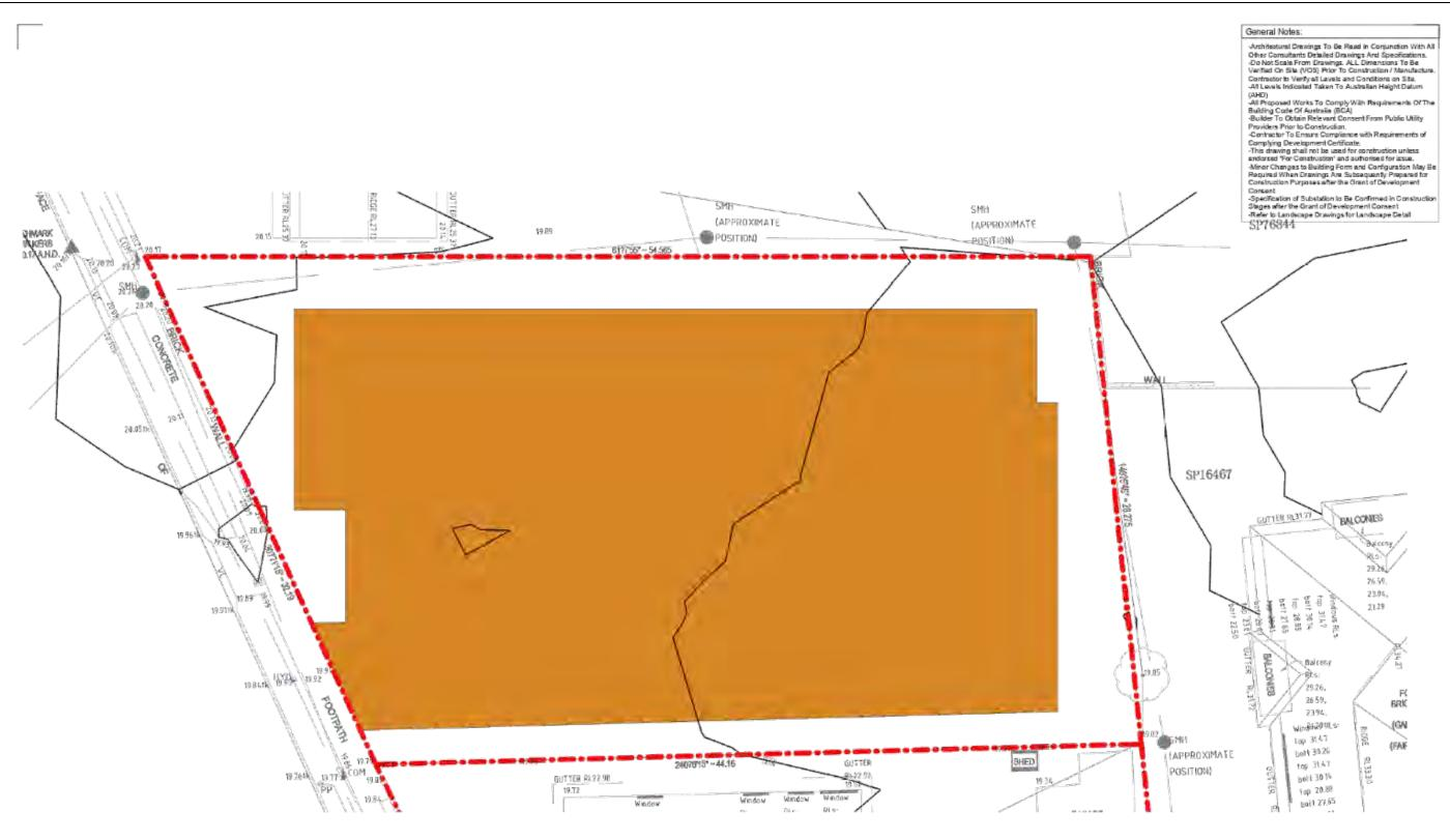
Average Approx. Excavation Depth: 3.6 m Approx. Excavation Volume: 3632 m3
