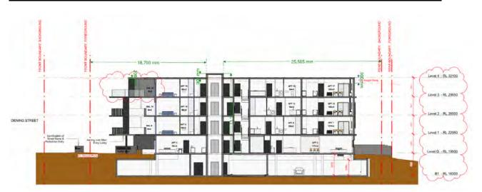
**Above: Section showing height breach**
