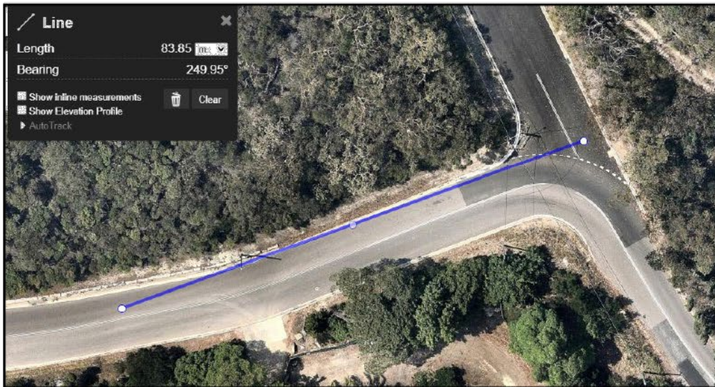
Figure 2 – Sight line for drivers exiting Debenham Road South onto Gindurra Road (source: Nearmap)
