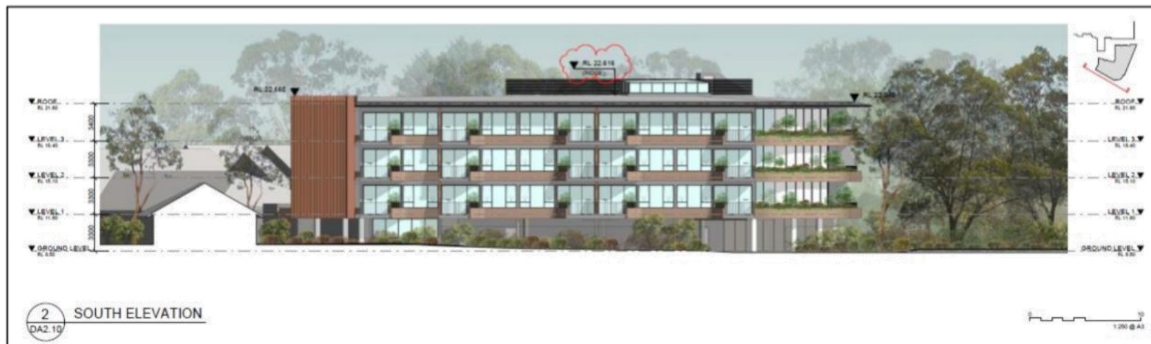
Figures 3 and 4 – North and South Elevations prepared by Marchese Architects showing the maximum height of the building as RL 22.560m and RL 22.616, which – when compared to a ground level of RL 8.5m – equate to encroachments of 27.85% and 28.32% respectively
