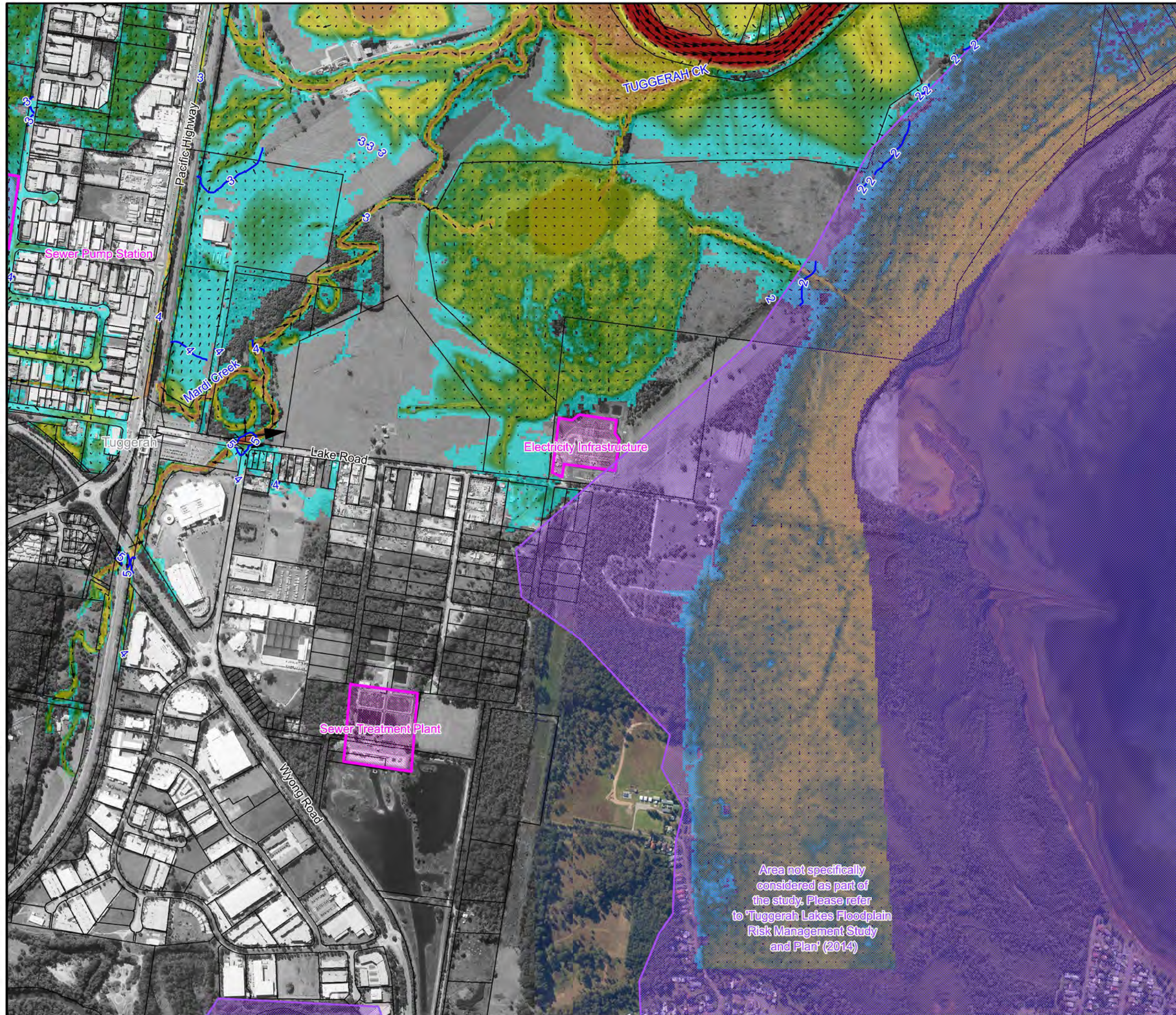
Figure A2.29: Peak Floodwater Depths, Velocities and Levels for the 5% AEP Flood
