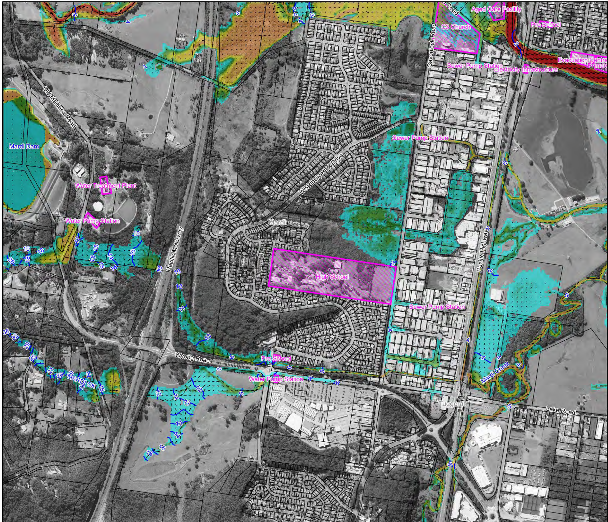
Figure A1.26: Peak Floodwater Depths, Velocities and Levels for the 20% AEP Flood
