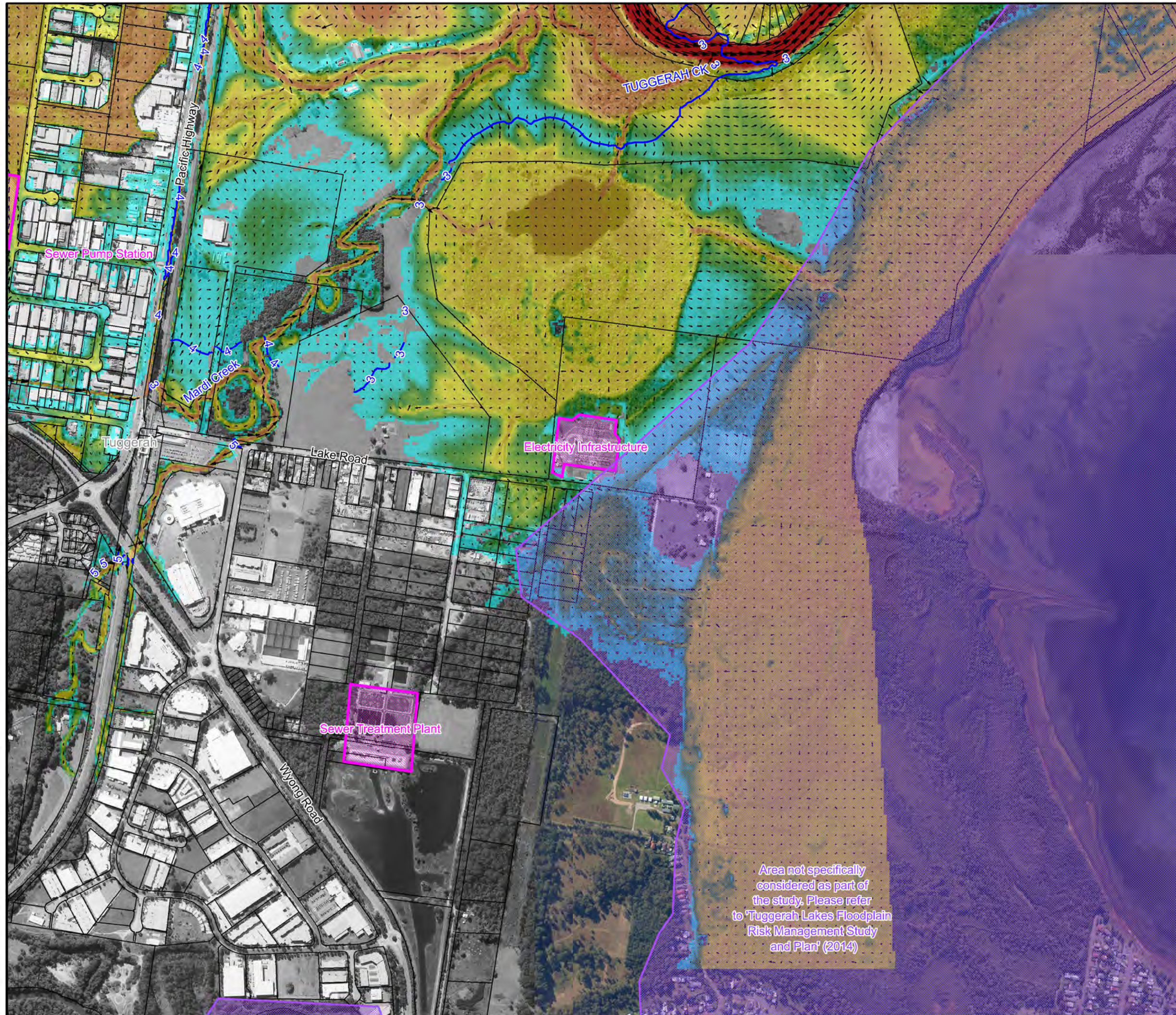
Figure A3.29: Peak Floodwater Depths, Velocities and Levels for the 1%AEP Flood
