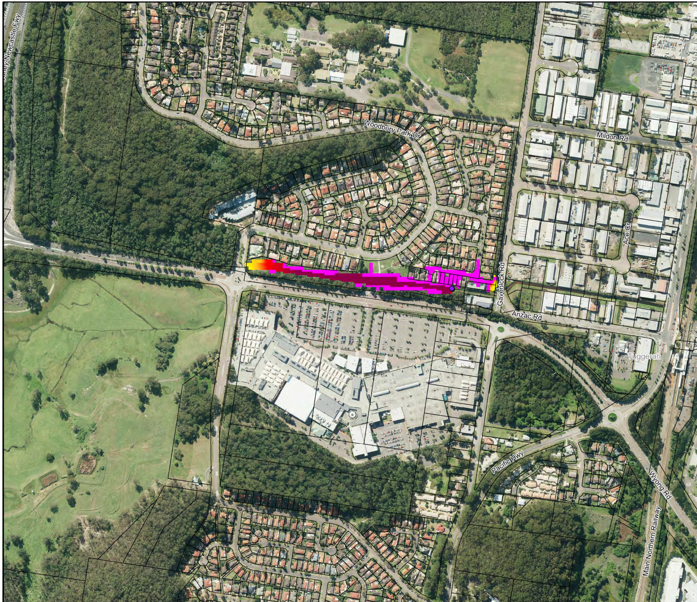
Figure G5: Flood Level Difference Mapping for the 1% AEP Flood with Debris Control Structures
