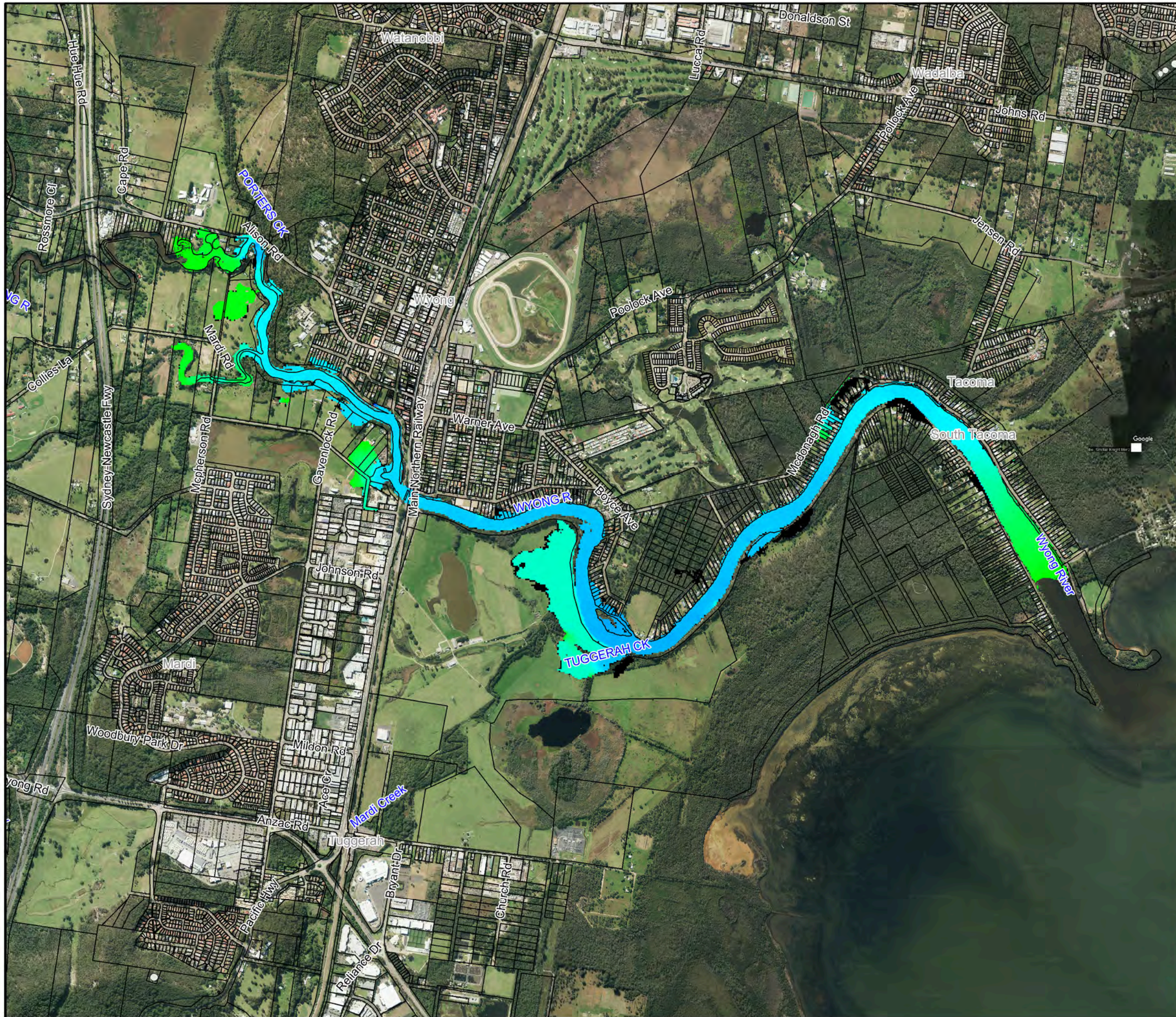
Figure H4: Flood Level Difference Mapping for the 20% AEP Flood with Dredging
