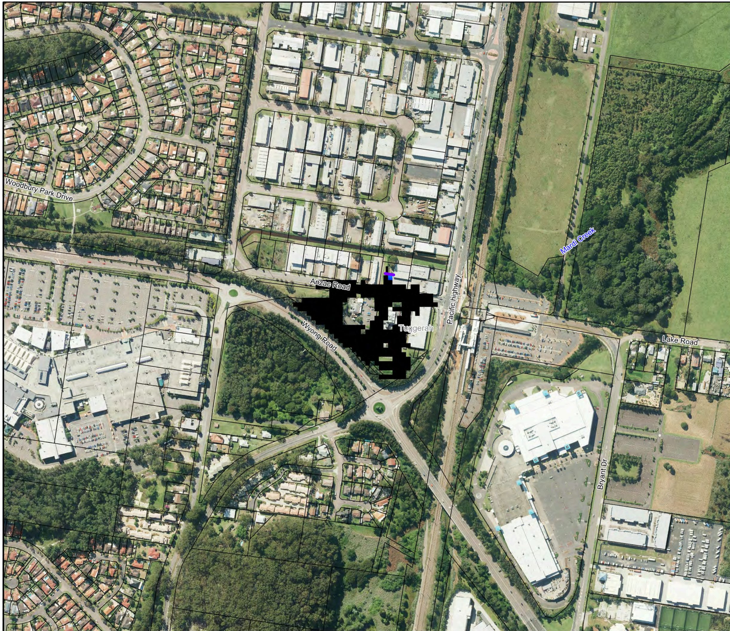
Figure C4: Flood Level Difference Mapping for the 20% AEP Flood with Anzac Road Levee
