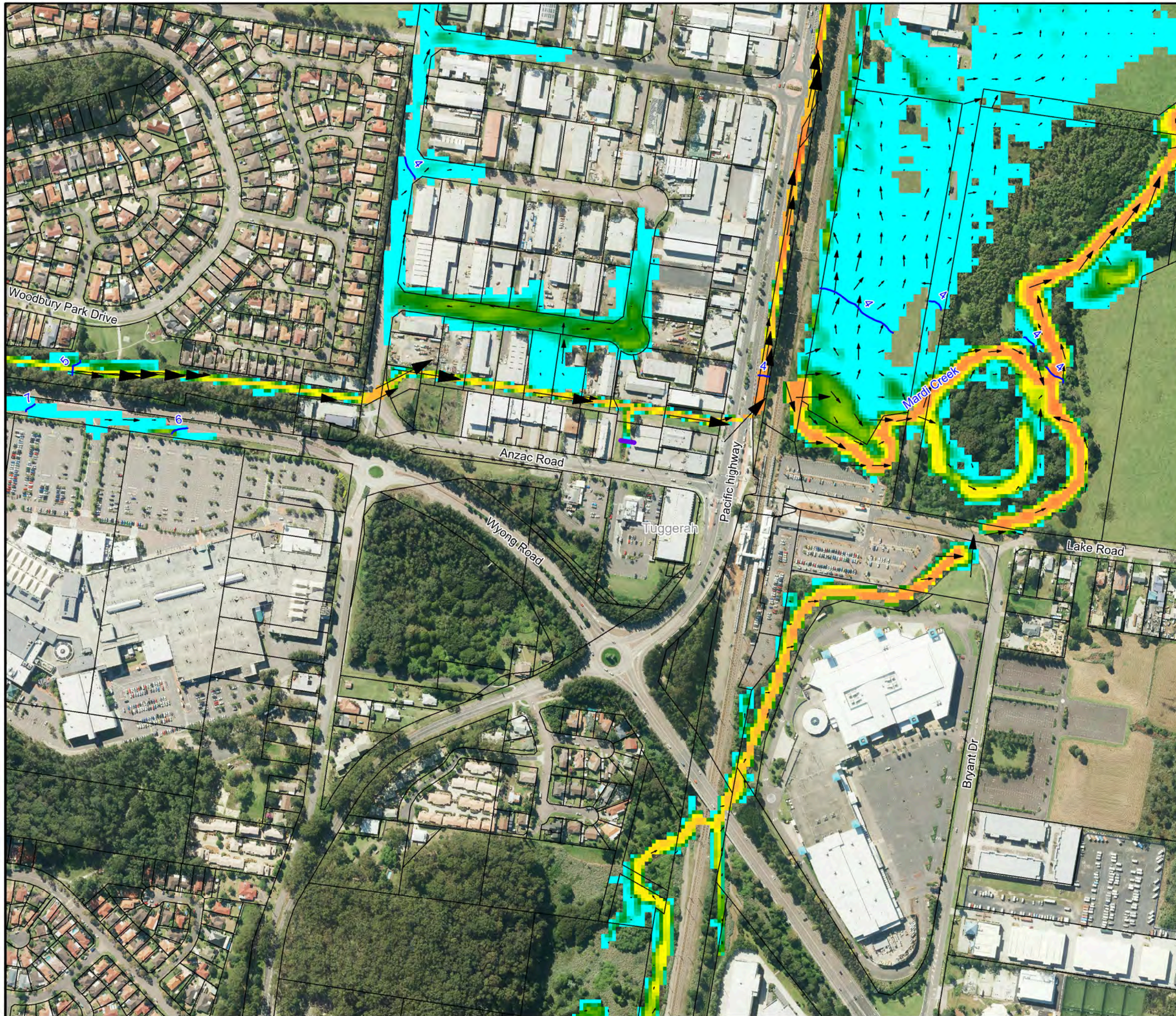
Figure C2: Peak Floodwater Depths, Velocities & Levels for the 20% AEP Flood with Anzac Road Levee
