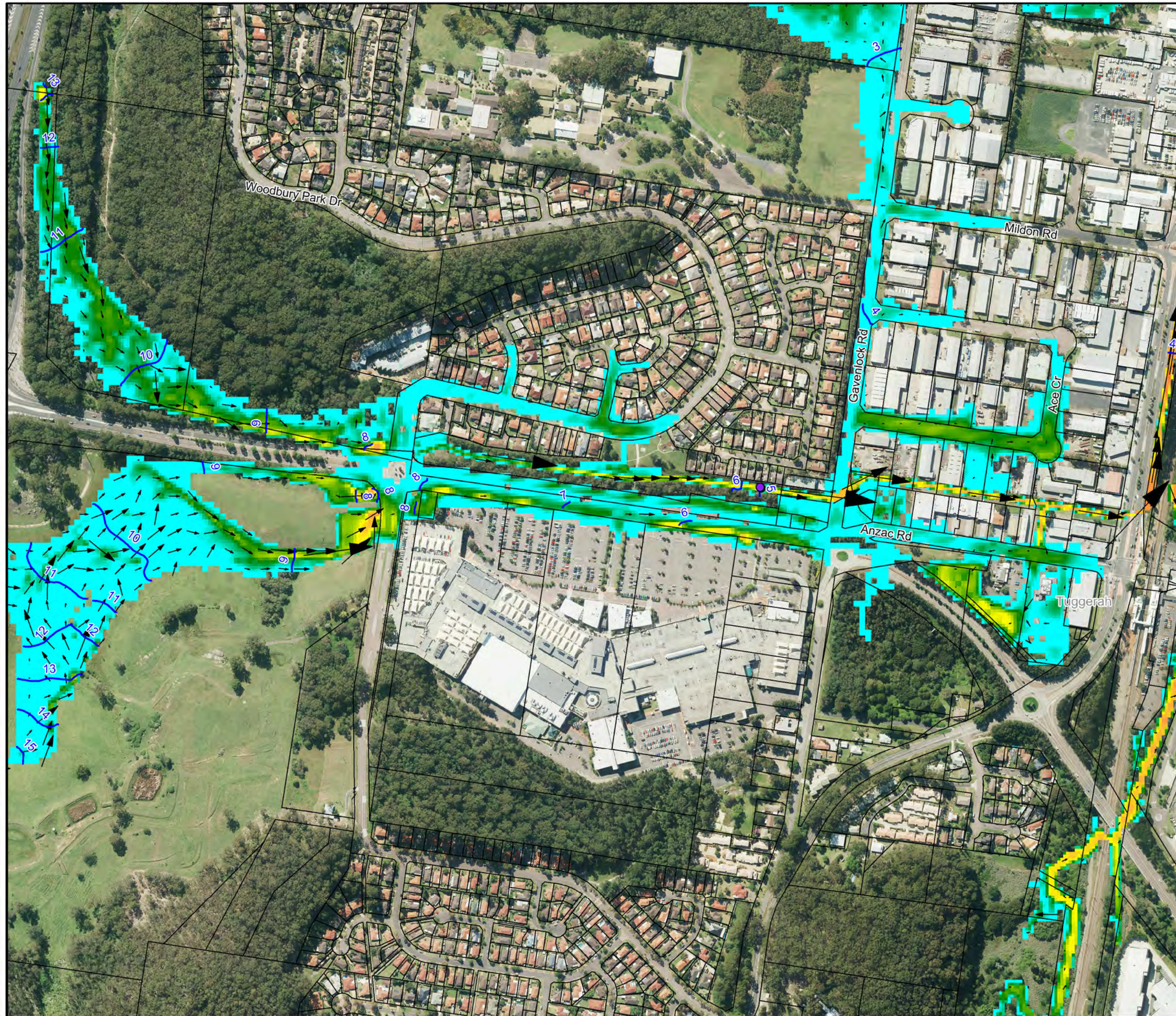
Figure G2: Peak Floodwater Depths, Velocities & Levels for the 20% AEP Flood with Debris Control Structures
