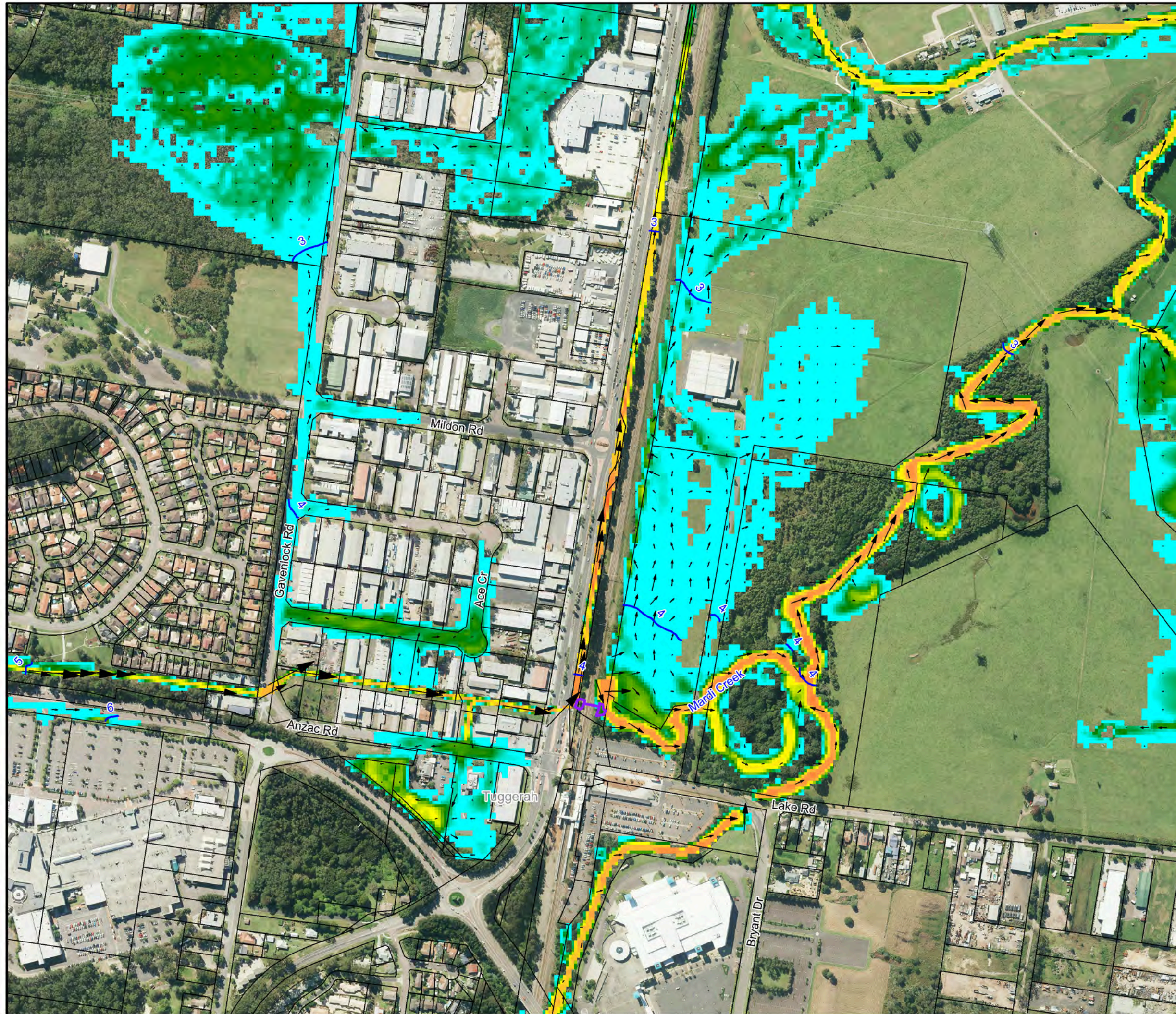
Figure D2: Peak Floodwater Depths, Velocities & Levels for the 20% AEP Flood with Mardi Creek Floodway
