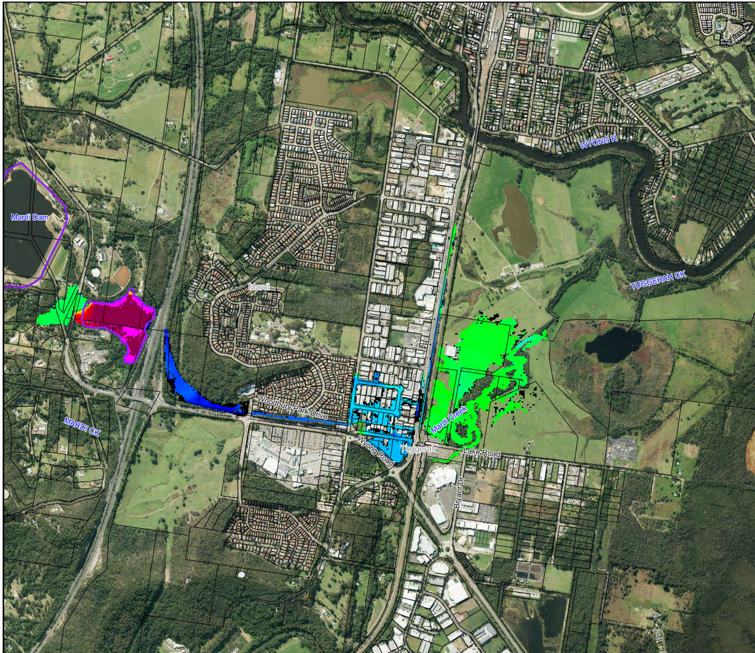
Figure B5: Flood Level Difference Mapping for the 1% AEP Flood with Mardi Creek Detention Basin
