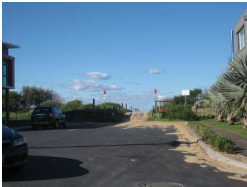
Figure 40: Potential for sand from beach to be lost onto the road by wind erosion
