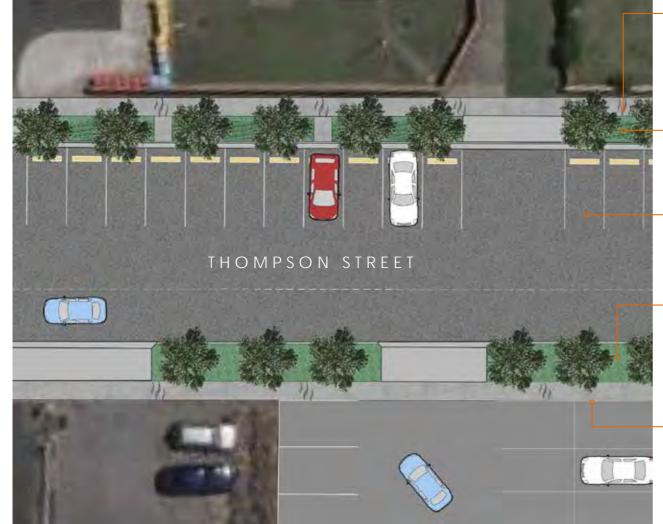
Existing 1200mm concrete footpath to be made good. Proposed shot blast pattern to be incorporated into existing concrete to future detail.
