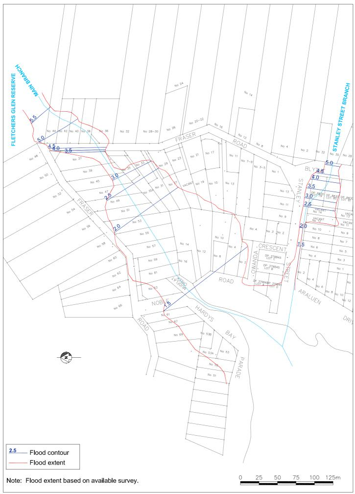
FIGURE 18 DESIGN FLOOD EXTENTS - 1% AEP + 0.5m FREEBOARD
