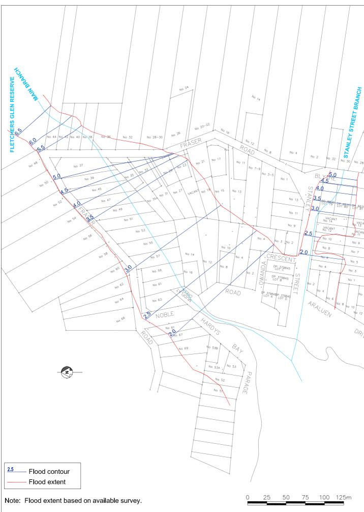
FIGURE 15 DESIGN FLOOD CONTOURS - 0.5% AEP CONDITIONS
