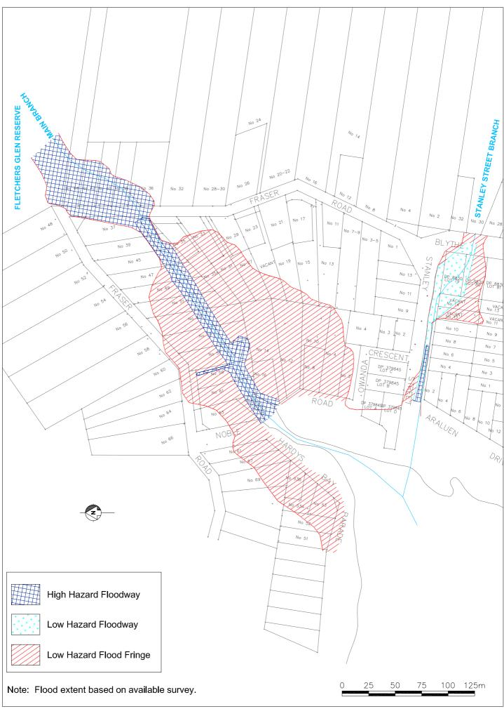
FIGURE 14 DESIGN FLOOD CONTOURS - PMF CONDITIONS
