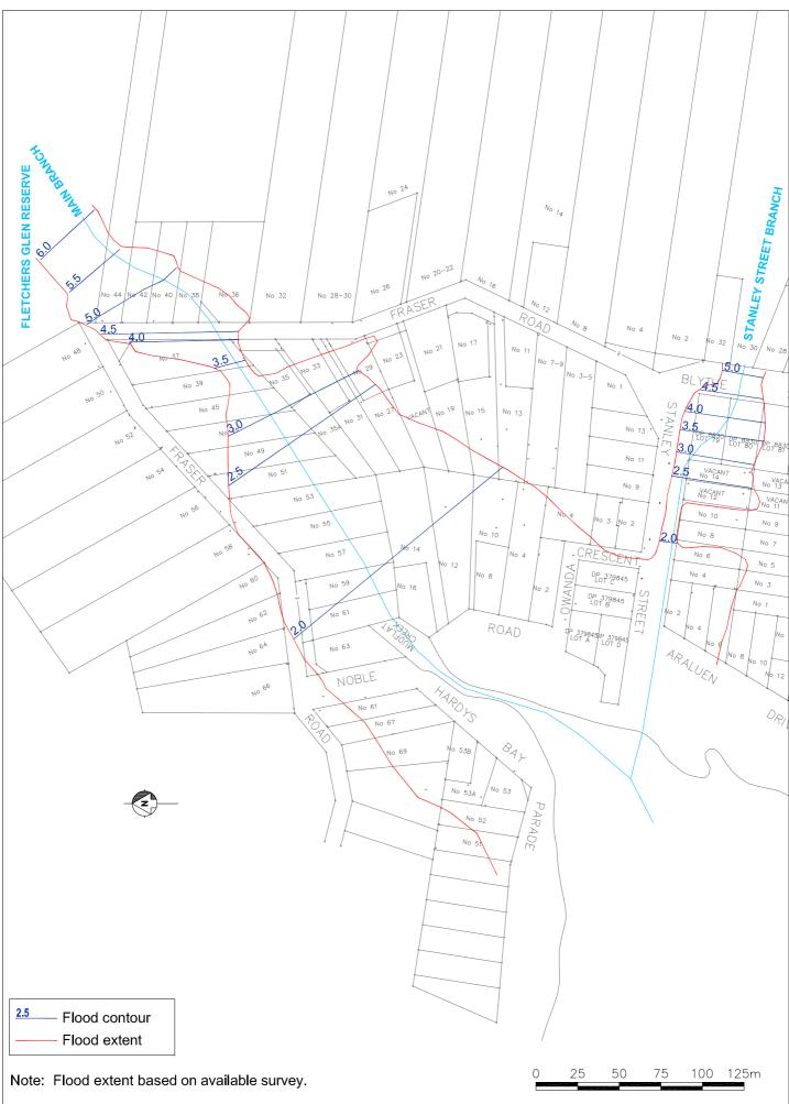
FIGURE 16 DESIGN FLOOD CONTOURS - 1% AEP CONDITIONS
