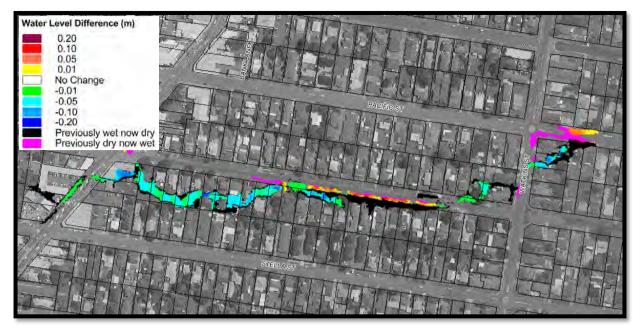
Plate 29 Peak 20% AEP Flood Level Difference Mapping with Kerb and Gutter installed along Elsiemer Street and Pacific Street
