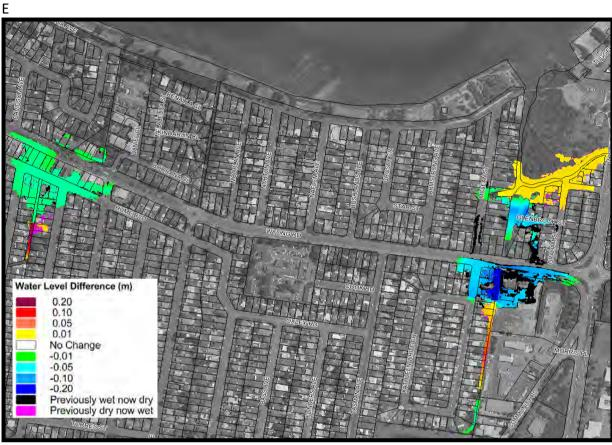
Plate 17 Peak 1% AEP Flood Level Difference Mapping with Blockage Control Structures
