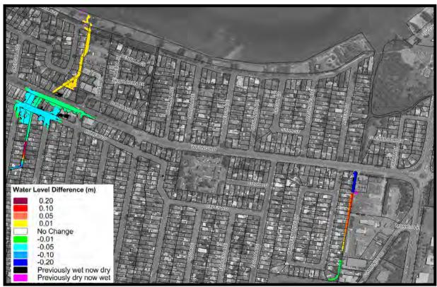
Plate 16 Peak 20% AEP Flood Level Difference Mapping with Blockage Control Structures
